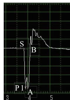
Figure 18 Waveforms with a transmitting 2 [MHz] and receiving 5 [MHz] probe.
