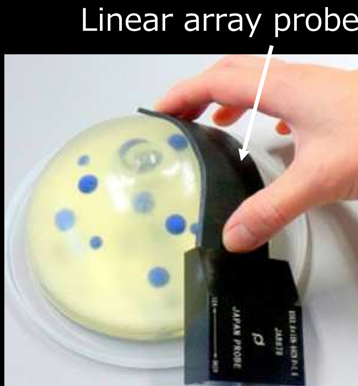
Flexible matrix array probe 8x8 64ch 2.5 mm pitch
