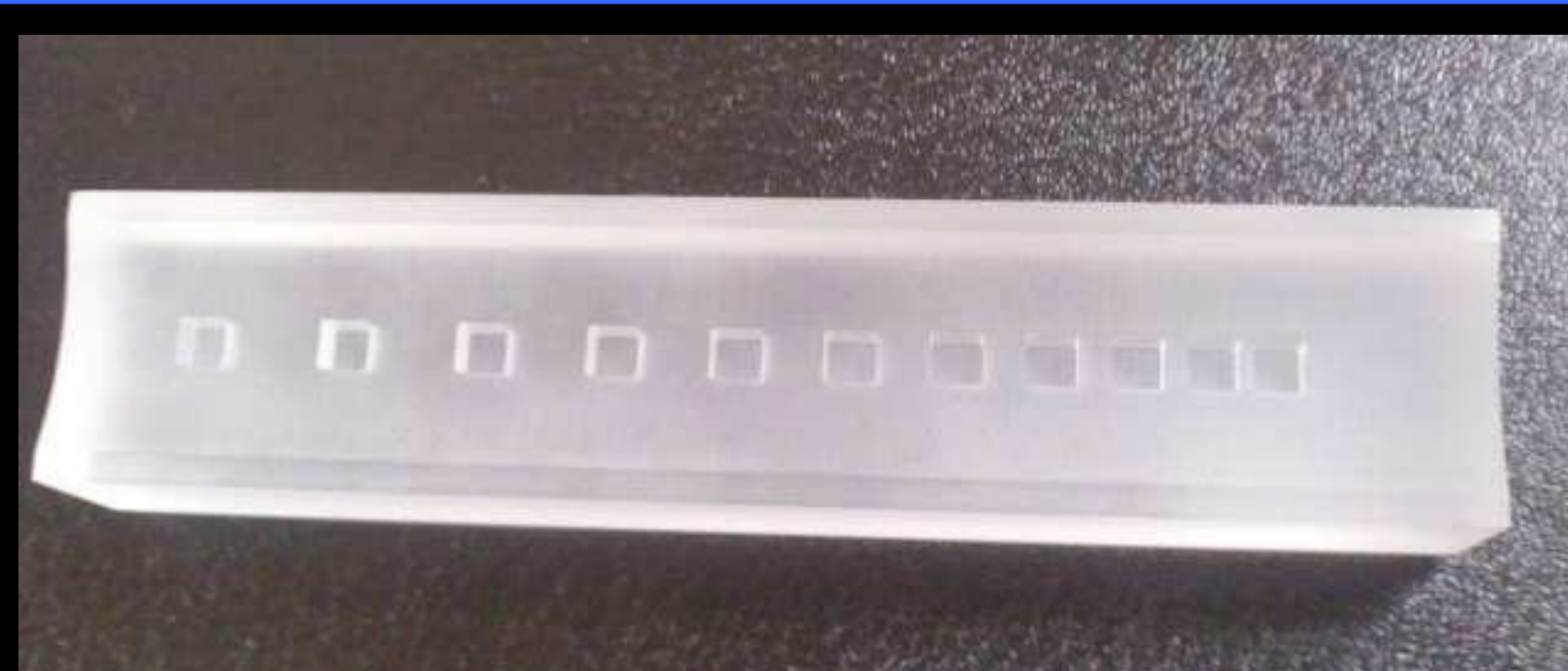
□5mm and □4 mm depth thinning 1-10 mm between each thinning
