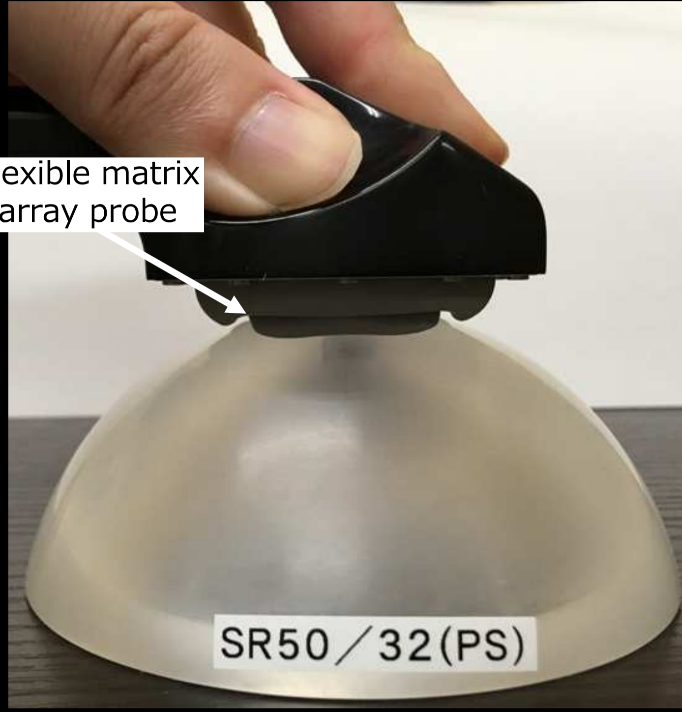
Flexible matrix array probe 8x8 64ch 2.5 mm pitch
