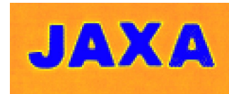
Test result image (C-Scope) by non-contact measurement in the air
