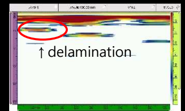
Example of a delamination 2mm under surface of CFRP
