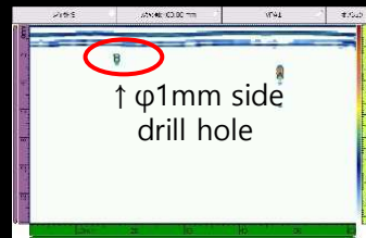
Example of a defect of \phi 1mm side drill hole 1.5mm surface in steel
