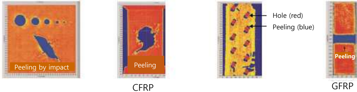
(Left: Image after impact test, Center: Image after lightning strike test, Right: Image after tensile test)
