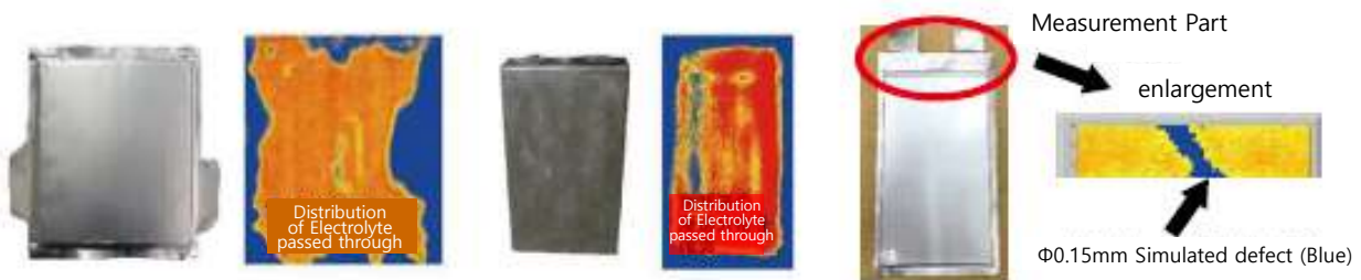
LiB (Lamination type) LiB (Square type) LiB (seal part of Lamination type) (Left: Specimen, Right: Image by NAUT21) (Left: Specimen, Right: Image by NAUT21) (Left: Specimen, Right: Image by NAUT21)
