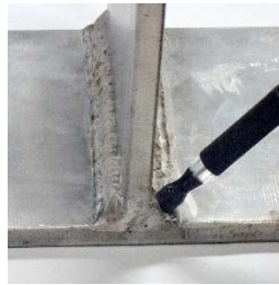
Fillet welding part
