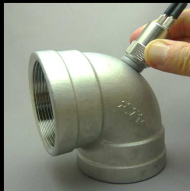
Thickness measurement of Elbow Pipe
