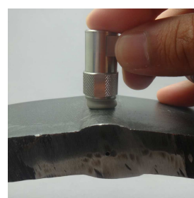
Inspection of Weld Bead (longitudinal)
