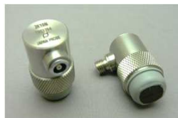
Single element straight beam type
