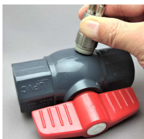
Thickness measurement of Valve
