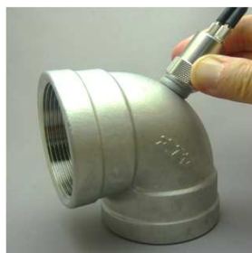
Thickness measurement of Elbow Pipe
