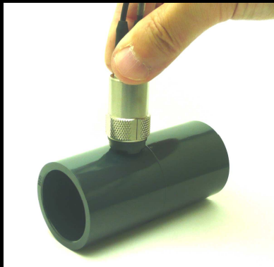
Example of Piping Thickness measurement ( t = 4\text{mm} )
